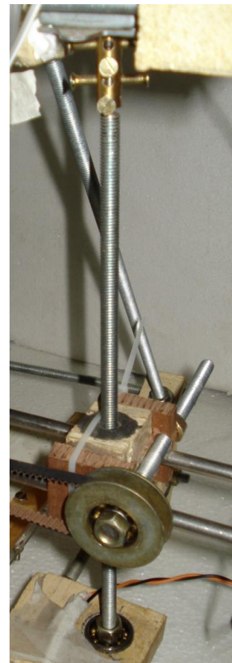
Fig 2.9: Z-Axis Lead screw assembly on the FDM machine
