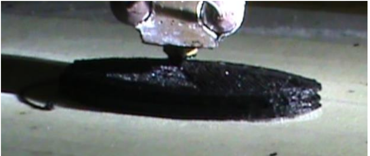
Fig 5.9: 8 th layer Infill
