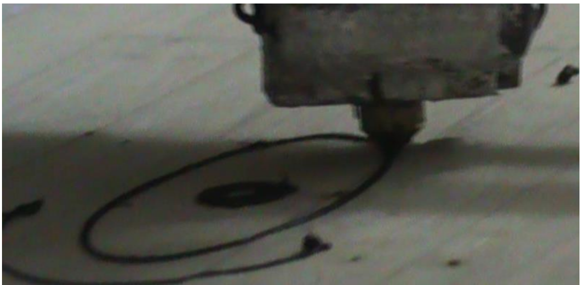
Fig 5.2: The first layer begins with the inner perimeter and extends outward. Here you can see the first perimeter completed.
