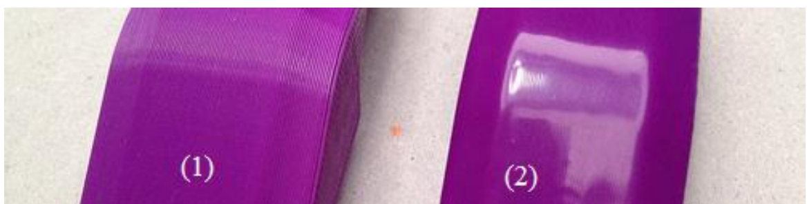
Fig 5.13: Acetone polishing. Notice the difference in surface finish of the two products.
